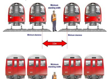
The ten foot / area between tracks can be used as a place of safety on:
