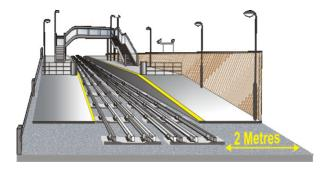
The track is not just the permanent way — but also the ground within 2 metres of any rail (unless guarded by an approved physical barrier) and platform ramps, but not station platforms.
