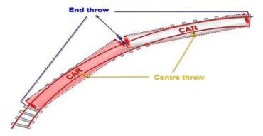
On curved track you should allow for extra clearance. This will depend on whether the track involved has a check rail.
