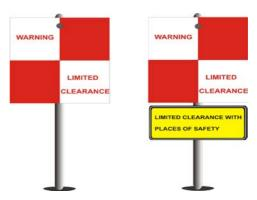
A limited clearance sign indicates a location besides the permanent way where a person cannot stand safely when trains pass.
