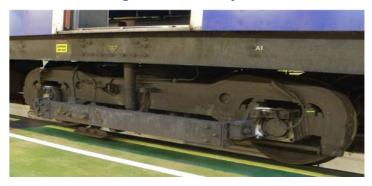
Collector shoes and the associated equipment may be live, even when not in contact with the conductor rails, therefore additional care must be taken to make sure that nothing worn or carried can touch the shoe gear when walking along the side of a train.
