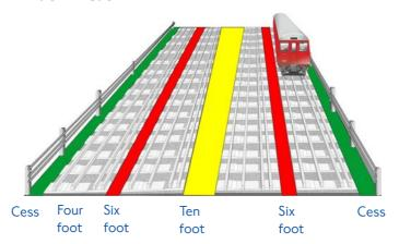
Cess - the space alongside the permanent way extending to a cable run or other boundary
